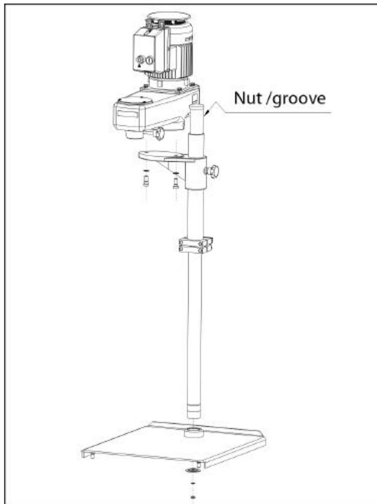
The stand pillar is inserted into the baseplate so that the guide groove is at the back. The black handwheel bolt is then on the right. The stand pillar is then secured from below with a hexagon nut, toothed lock washer and a large shaped washer.
