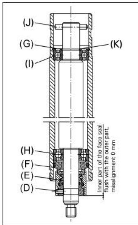
To change the slide ring seal and the ball bearings, proceed as follows:
