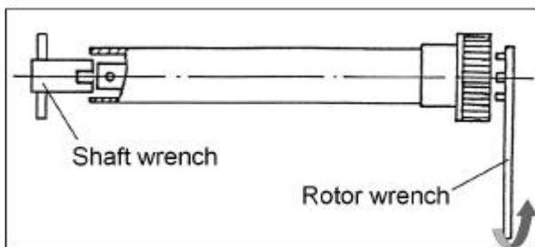
The stator can be very tightly seated on the shaft tube, particularly when working with viscous substances, or when cleaning has been neglected, or when medium has penetrated into the thread between shaft tube and stator. In this case, the shaft tube can be held in a vice with soft jaws to crack the thread. Note the left-hand thread!
