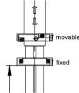
Fix item 4 on the stand pillar for the desired switch-off height
