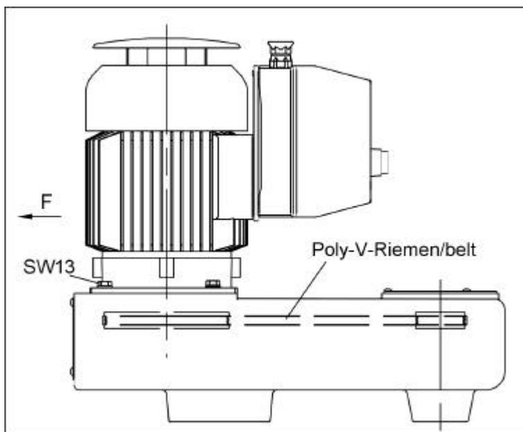
1. Slacken off the four hexagon head bolts near the motor using a 13mm a/f wrench.
