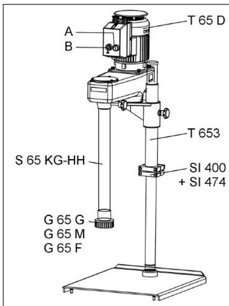
For operation, the T 65 D dispersion unit must be mounted on the IKA® T 653 telescopic stand. It must only be operated with the S 65 KG-HH shaft and the dispersion tools from the S 65 range (G 65 G, G 65 M, G 65 F). The unit is switched on and off by pressing the ON button (A) and the emergency stop button (B). If the emergency stop switch of the dispersion unit is not within reach, an additional emergency stop switch must be installed within easy reach, in the working area.
