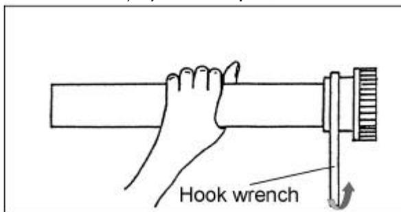
3. Screw the rotor clockwise on to the shaft (right-hand thread). To do this, hold the shaft with the shaft wrench at the coupling section and tighten the rotor with the rotor wrench. With the G 65 G generator, the rotor wrench is inserted between the teeth of the stator and turned.
