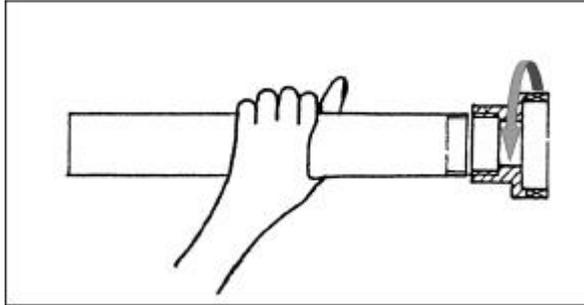
2. Gently tighten the stator with the hook wrench. The stator is turned in the same direction later, by the flow pressure of the rotor, and hence cannot come loose.
