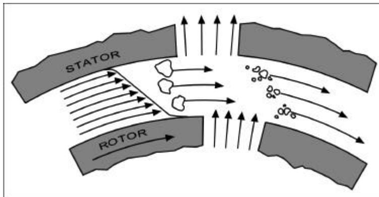
The dispersion effectiveness is heavily dependent on the product of the shear gradient and the time the particles spend in the shear zone. The optimum range for the circumferential velocity of the rotor/stator arrangement is 10 to 24 m/s.
